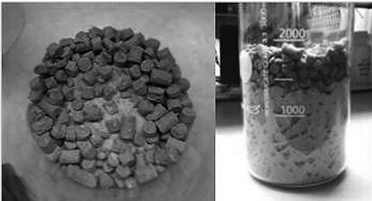
Figure 1. Emplacement of the bimodal blend in laboratory
